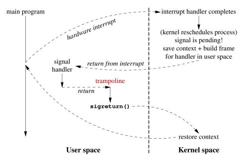
The kernel uses the signal trampoline to arrange that control is bounced back to kernel after execution of signal handler
